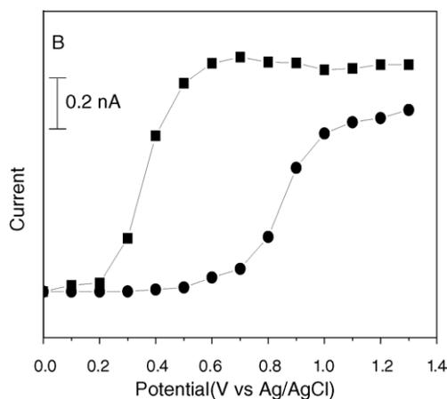
Fig. 2. Hydrodynamic voltammograms for  $200 \mu\text{M}$  *p*-aminophenol (■) and  $200 \mu\text{M}$  acetaminophen (●). Conditions—separation voltage: 1800 V; sample injection: at 1000 V for 5 s; working electrode: Pt ultramicroelectrode; running buffer: acetate buffer (10 mM, pH 5.0).
