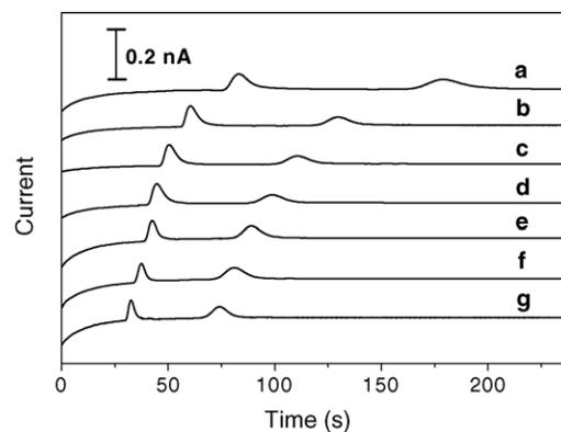
Fig. 3. Influence of separation voltage on the electroperograms. Separation performed at (a) 800 V; (b) 1000 V; (c) 1200 V; (d) 1400 V; (e) 1600 V; (f) 1800 V and (g) 2000 V. Other conditions as in Fig. 2.
